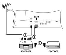
Connect the aerial cables ①, ② and, to obtain the optimum picture quality, eurocable ③ as shown. If your recorder does not have a euroconnector, the only possible connection is via the aerial cable. You will therefore need to tune in your recorder's test signal and assign it programme number 0 or store the test signal under a programme number between 90 and 99, see Manual installation, p. 6.
